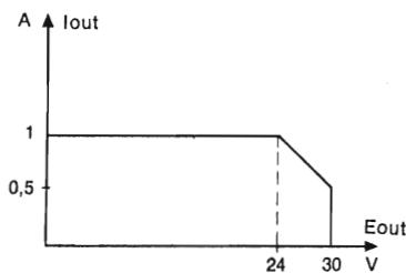
The power supply TPS 1d can be used as constant voltage source as well as constant current source.
